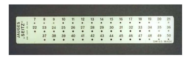
If you have no pivots, you could measure the inside diameter of the balance hole jewels ("0.12" is 0.12 mm.):
