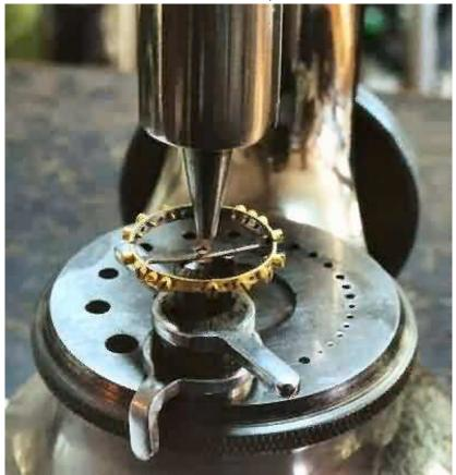
Measure the diameter of the pivot. A pivot gauge like this one makes this measurement easy ("12" is 0.12 mm.):
