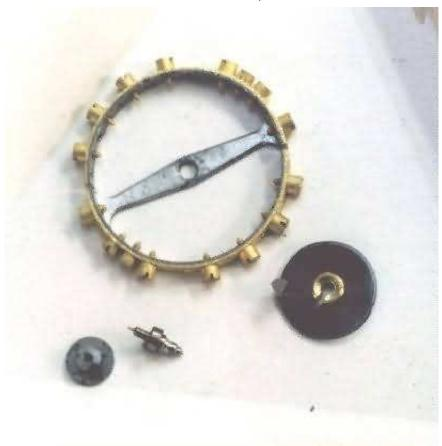
Place the new staff into a hole in the staking block, where the hole just fits around the staff, with the small shoulder just above the staff hub facing upwards. Place the balance wheel onto this hub shoulder and stake the shoulder over the edge of the balance using a round-edged hole punch first, to spread the shoulder, and then a flat-faced hole punch to "fold" the edge of the shoulder over the balance.
