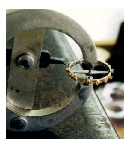
The roller table is installed under the balance wheel against the hub using the staking set. If the roller is a single roller, you must select a hole punch with a notch on the side for the roller jewel. This watch has a double roller, however. You must align the roller jewel with the marking you made on the balance wheel earlier. After staking on the roller table, you must check the poise (weight distribution) of the balance assembly, without the hairspring:
