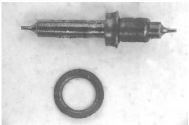
The balance and staff are mounted onto a hole stump (part of the staking set) with the hairspring side facing down. A hole punch with rounded edges is mounted through the hole at the top of the stake and over the end of the staff pivot. A small amount of tapping with a one-ounce hammer and the balance staff should fall out easily.
