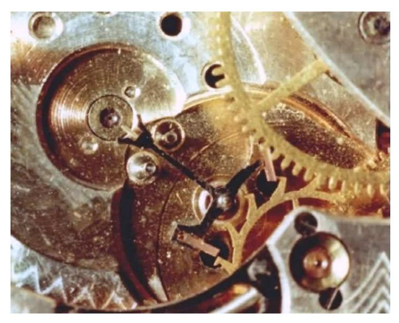
After marking the positions of the roller jewel and the hairspring stud on the balance wheel (you could use a felt tip pen that could be cleaned off later), the hairspring is removed by using a pair of miniature tools for this purpose. For clocks and pocket watches, two of the smallest watchmaker's screwdrivers would work well to remove the hairspring, but this must be done very carefully! To remove the roller table, a nice staking set like this one serves the purpose:
