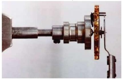
The pivot on the left side has obviously broken off and the other pivot appears to be bent:
