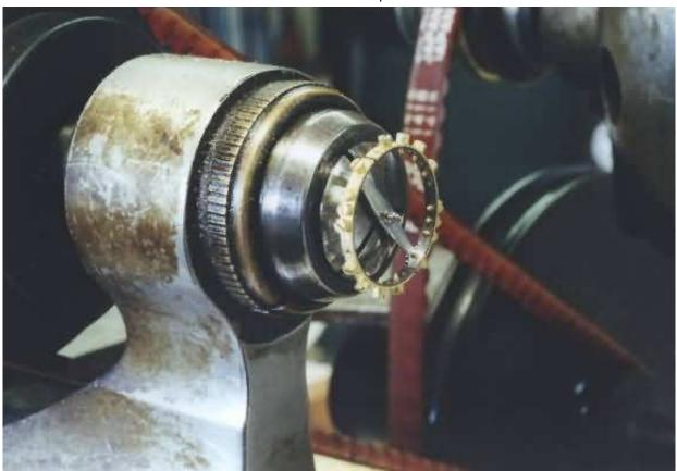
Use a graver to remove the hub on the staff. This is a steel graver (a carbide graver is much better for this purpose):
