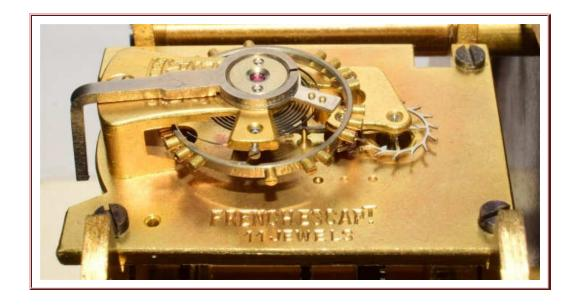
Smiths clock began production of a clock with a newly designed "floating balance" by Hettich of Germany, in 1956. Notice that the balance wheel also moves back and forth on a horizontal plane. I have several of these Smiths K7A clocks, manufactured in Wales in 1959, and they have an accuracy similar to the Elliott. The Smiths K7A floating balance clock was effectively a major upgrade to the Smiths K6A pendulum clock that came before it.
