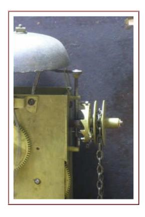
The escape wheel moves the pallets back and forth, causing the hammer to move back and forth, striking the bell. Here you can see the alarm hammer with the bell removed, and this is where the enormous significance of the alarm mechanism for the evolution of timekeeping becomes clear: if you add another hammer on the other side, you have a foliot. The earliest known mechanical clock was from around 1285, according to church records.
