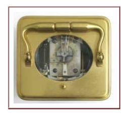
Around 1950, an Elliott clock was produced with a l'Épée escapement platform, like the one below from the 1960s. It has the same platform used on carriage clocks. These clocks were far more accurate than the average mechanical clock at the time, with an error of only about a minute per week. However, the Elliott clock was very much a luxury item: it was a very
