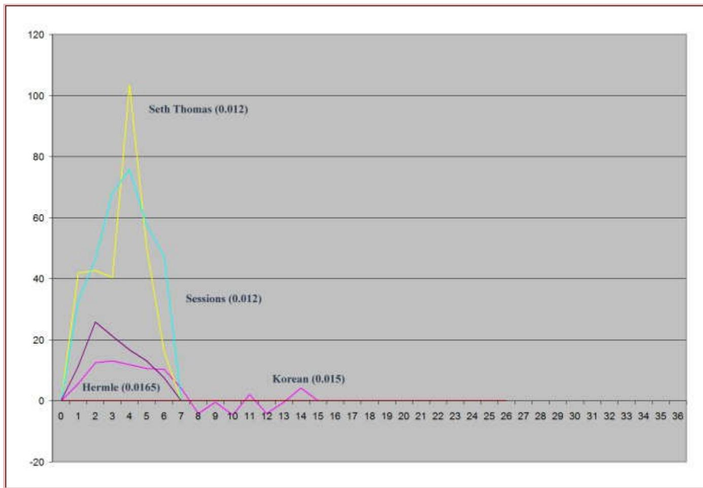
The data for the 31 day clock shows more clearly than for the other clocks how accuracy can be improved by winding the clock twice per cycle. If you have a clock which you wind once a day, wind it twice a day. If you have a clock which you wind once a week, wind it twice a week. If you have a clock which you wind once a month, wind it twice a month. Every time you wind your clock, move the minute hand a minute or two to the correct time.
