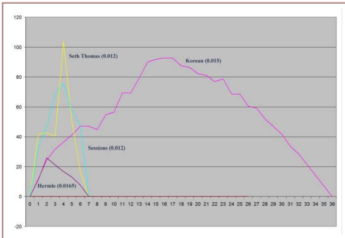
Considering a normal 31 day run, an overall error of 75 seconds over 31 days is very respectable for a spring-driven clock. This clock gained 5 seconds per day during the first half of the month, and lost 5 seconds per day during the second half of the month. Few clocks can match that performance. The clock could be made more accurate by winding it twice a month. The overall error would be reduced from 75 seconds to 13 seconds.
