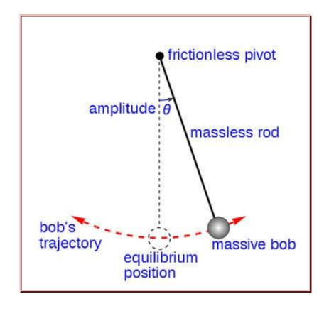
The moment a pendulum is released, gravity pulls it straight down, and a portion of that pull acts to pull the pendulum towards its vertical position, depending on the angle, the length of the pendulum, and the force of gravity, given by the following equation, in which acceleration is theta with an umlaut (two dots) over it:
