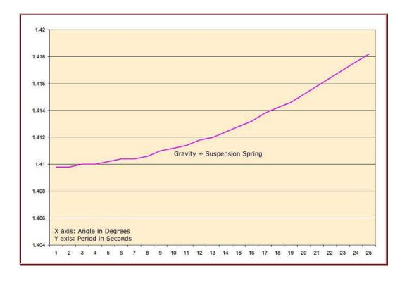
However, the coefficient of elasticity is NOT constant for larger angles. For example, if you double the angle from 45° to 90°, the force the suspension spring applies increases, but it does not double. The line for the suspension spring in the graph above should therefore curve upwards some as the angle increases.
