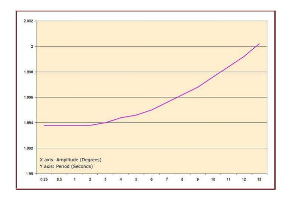
The graph shows that the period reaches two seconds when the angle reaches  $13^{\circ}$ . This means that the period is less than two seconds for smaller angles, causing a clock to gain time, but greater than two seconds for larger angles, causing a clock to lose time as a result of circular error. Notice that, for small angles, of  $3^{\circ}$  or less, the curve becomes flat because of what is called Linearization (when  $\sin\theta$  is approximately equal to  $\theta$ ).
