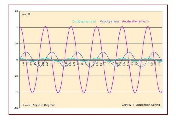
Peak velocity increases by 41%, but displacement remains unchanged.
