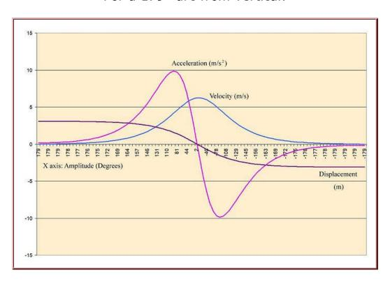
Looking at several graphs below, we can see that, as the angle increases, the height (amplitude) of the acceleration curve increases, but at a declining rate: when the angle doubles, the acceleration increases by less than double.
