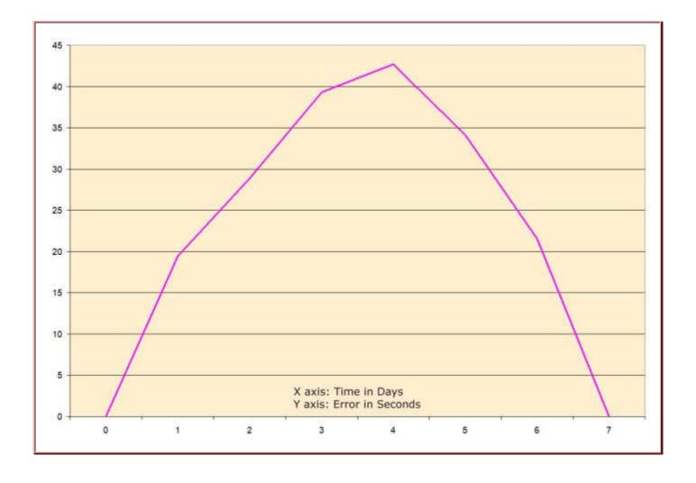
If you adjust the pendulum such that the clock keeps accurate time for the first four days, and wind the mainspring twice a week, you will notice a big improvement in overall accuracy. In this example, the peak error goes down from 43 to 9 seconds, a decrease of 79 percent.
