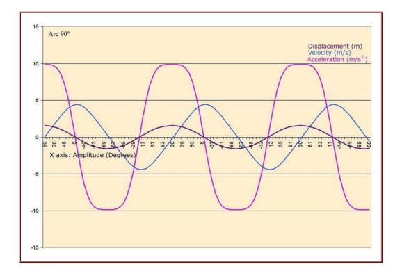
Beyond 90°, the acceleration curve no longer reaches a higher high, and forms what looks like a wave within a wave.
